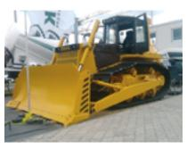
TM10 bulldozer with new hydrostatic power transmission (Bosch-Rexroth HST) was commercialized. The selection of such HST is explained by successful utilization of this transmission by the leading manufacturers: Liebherr, CAT, Komatsu, John Deere, CHETRA. The main units are welded with KAWASAKI and MOTOMAN.
